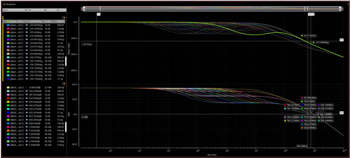
Figure 2.4: Effect of varying R_c and C_c
