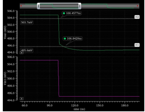
Figure 3.11: Annotated 10-90% time (505 mV–495 mV)
